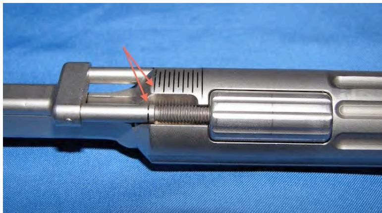
The arrows show the Stop too far forward. This setting may cause the Stop to be tightly bound by the Trial head when attached and the knob will not be able to be moved. Remove the Trial and adjust the Stop to a position behind the first mark on the handle.
