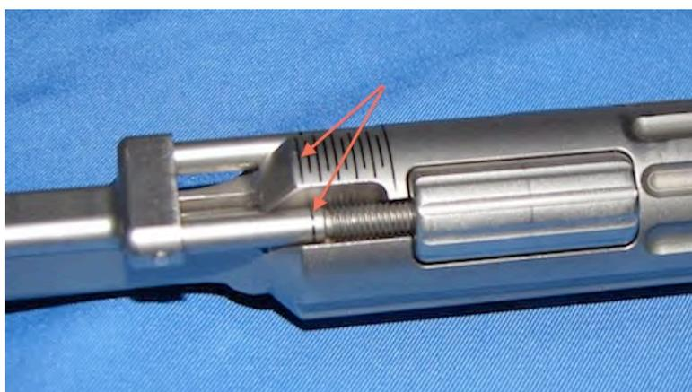
The arrows show the best position to start. To prevent any chance of binding, make sure the Stop is not set any farther forward than this position before attaching the Trial to the Handle.
