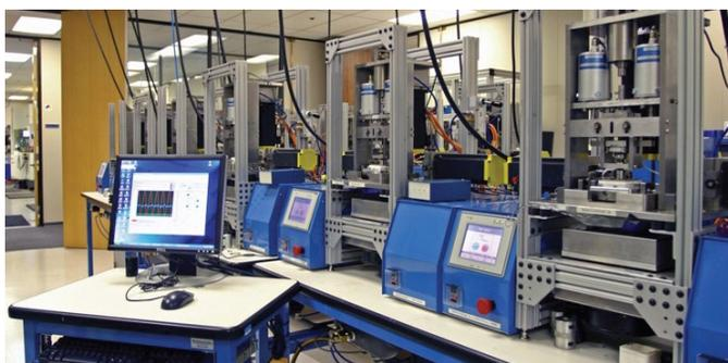
Figure 1: Functional kinematic testing was conducted using custom-built machines designed by Spinal Kinetics.
