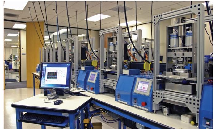
Figure 1: Kinematic wear testing was conducted using custom-built machines designed by Spinal Kinetics
