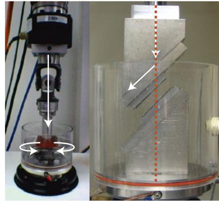
Figure 2: Static and Dynamic testing. Left: Compression and Torsion. Right: Compression Shear.
