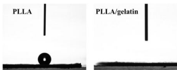
Figure 5. Water droplet image (2 s recording) on PLLA membrane and PLLA/gelatin membrane.
