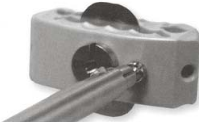
Screwing of the safety screw
